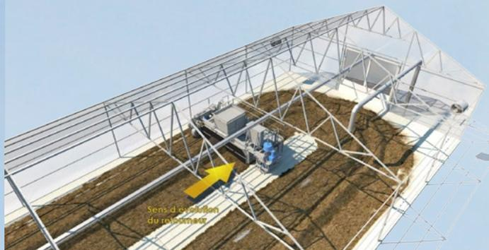
*The innovation brought by Veolia's SOLIA Mix solar sludge drying comes from using a completely new design of windrow turner.*
